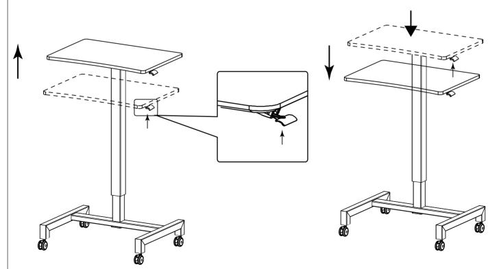
Lift the paddle for lifting the table top.
